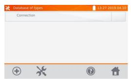
The meter has default types saved in its memory. Use  $\bigoplus$  icon to add a new type of the tested object.
