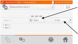
Auto/Manual switching (auto / manual range selection): **Auto** - the measuring current is limited to a value not exceeding the set value, **Manual** - measuring current
