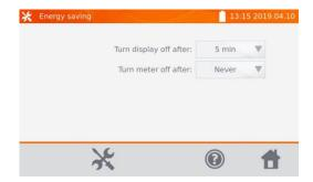
Set the inactivity time for blanking the screen and turning the meter off.
